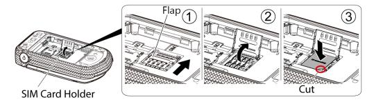
5. Lower the flap of the SIM card holder (4) and slide the flap in the direction of the arrow to lock it (5).
