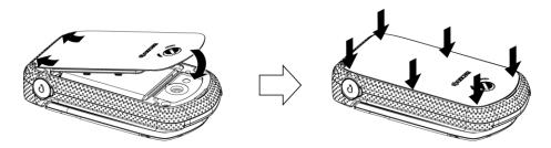
5. Using a coin, rotate the battery cover screw in clockwise direction until the cover locks.
